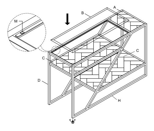
Adjust the Pre-installed Levelers height to achieve balance.
