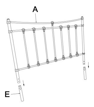
Assemble 4 pcs Bolt with ball (G) to the Headboard (A) and Footboard (B). Assemble the Side rail (C) to the Headboard (A) and Footboard (B) with 12 pcs Bolt (I), 8 pcs Nut (K) and 8 pcs Flat washer (L) by Allen wrench (M) and Wrench (N).
