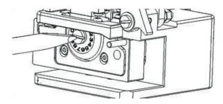
1. Unscrew the screw that connects the blade carriage sliding block.
