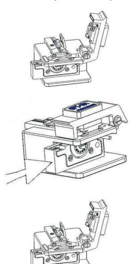
Preparing fiber involves removal of colored soft peel coating per instruction steps included with SSF™ connectors. Do not attempt to cleave fiber that has not been prepared.
