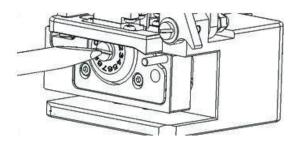
1. Unscrew the fastening screw of the blade, turning in a counter-clockwise direction with a screwdriver. Rotate blade by one postion to the next number (original number on blade plus one), then tighten screw.
