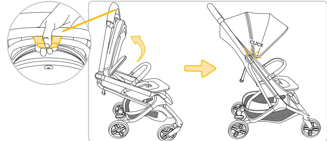
Locate the frame fold release buttons on the handlebar. Squeeze in the small button first and then squeeze in the larger button. While squeezing both buttons, unfold the stroller by pulling it up until it clicks into place.
