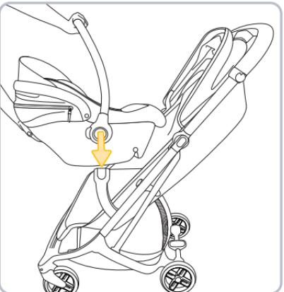
Lower the car seat onto the car seat adapters until it clicks into place. Once installed, pull up on the car seat either at the carry handle or at the handle hubs to check if it is securely attached.
