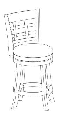
This page lists all the contents included in the box. Please take the time to identify the hardware as well as the individual components to this product. As you unpack and prepare for assembly, place the contents on a carpeted or padded area to protect them from damage. Attach the Chair Leg (E) to the Apron With Swivel Plate (D), then attach the Footrest (C) to the Chair Leg (E) using Bolt (F), Lock Washer (H) and Flat Washer (I) with Allen Wrench (K).
