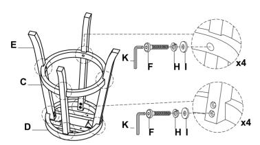
Take the Allen Wrench, and turn the bolts until the legs are secured. DO NOT TIGHTEN COMPLETELY. Stop when you feel you are adding force to tighten the bolt.
