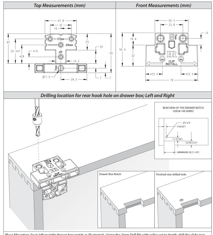
Place Mounting Jig in left or right drawer box notch as illustrated. Using the 7mm Drill Bit with collar set to depth, drill the slide rear hook hole. Repeat on opposite side.
