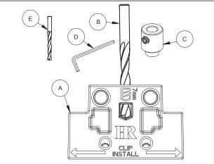
Place 7mm Drill Bit in set hold of jig as illustrated. Slide Drill Bit Depth Collar on Drill Bit and adjust it to set on the jig. Tighten allen set screw to secure collar.
