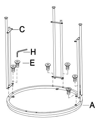
Attach Shelf Frame (B) to Leg (C) by Bolt (E) and Allen Wrench (H). Then attach Leveler (G) to the bottom of Leg (C) as shown.
