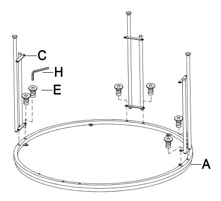
Attach Shelf Frame (B) to Leg (C) by Bolt (E) and Allen Wrench (H). Then attach Leveler (G) to the bottom of Leg (C) as shown.
