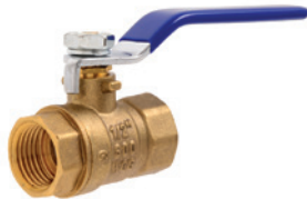
BALL VALVE, 400/600 W.O.G. NON-SHOCK (WATER, OIL, GAS) FULL PORT FEMALE PIPE TO PIPE
