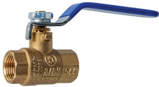
FULL PORT TWO WAY BALL VALVE, CGA 3.16, 600 P.S.I. LONG LEVER HANDLE FEMALE PIPE TO PIPE
