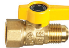
BALL VALVE, CGA 9.1 APPROVED FOR 1/2 PSIG TEE HANDLE MALE SAE FLARE TO FEMALE PIPE
