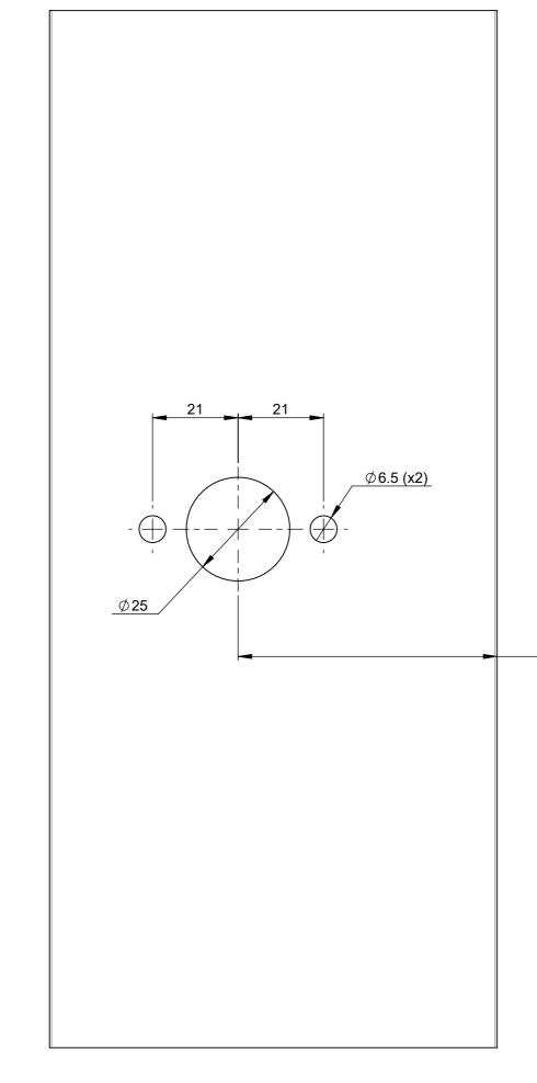
BACKSET MEASUREMENT FROM FRONT FACE OF FOREND ON LATCH OR LOCK.
