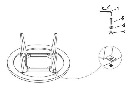
STEP 4 Tighten all Bolts with Allen Wrench #1
