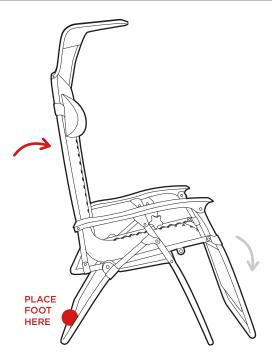
To return to an upright position, loosen the knobs, place a foot on the back chair leg, and push the backrest upright.
