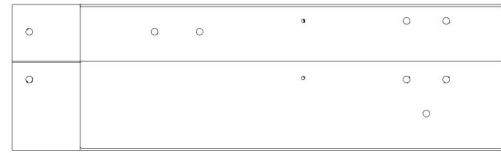
J08 JOIST ASSEMBLY - W2A03725 (x1) 1 7/16"x8 7/16"x28 7/16" (36x214x722)
