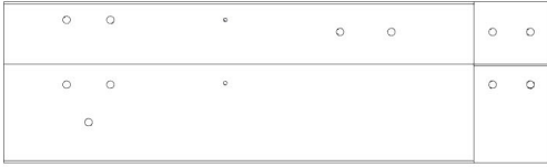
J10 JOIST ASSEMBLY - W2A03727 (x1) 1 7/16"x8 7/16"x28 7/16" (36x214x722)
