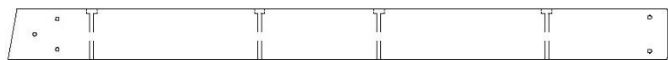
SB74 | POUTRE DE BALANÇOIRE 2 POSITIONS - W4L13291 (1) | 2 po x 5 1/4 po x 68 3/4 po (50x134x1745)
