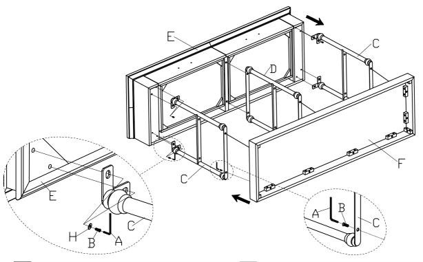
Assembly the Shelf(G) onto the Side Frame(C). then using the Bolt(B) by Allen Wrench(A).
