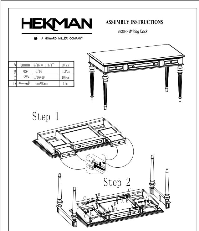
Step 1: Remove the end drawers - Open drawer fully to expose the release levers in the center of the drawer slide. Push the lever on the left side up, and the lever on the lever on the right side down to release drawer. With levers pushed gently tug the drawer out of the desk
