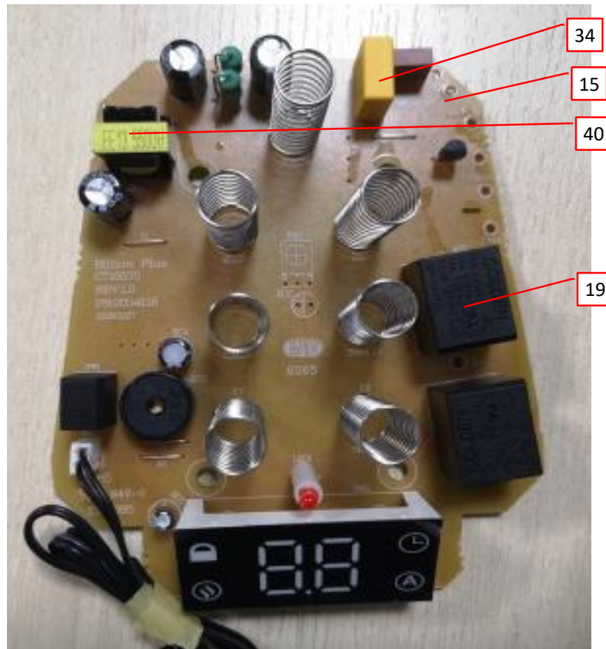
Photo 20 - PCB, Billion Plus, 2034116, Used in model CT16570
