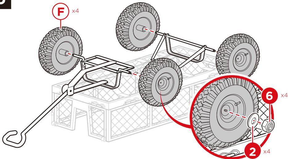
Insert four part F wheels into part J front axle and part B rear axle frame using a part 2 washer and part 6 nut for each wheel. Use the air pump to inflate the wheels to a maximum of 25 PSI.
