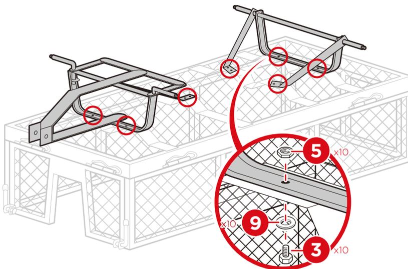
Attach the completed item from step 1 to part A bottom frame using six part 3 bolts, six part 5 nuts, and six part 9 washers.
