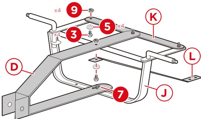
Use a part 3 bolt, part 5 nut, and part 9 flat washer to attach part D yoke, part J front axle, and part L front axle brace together.
