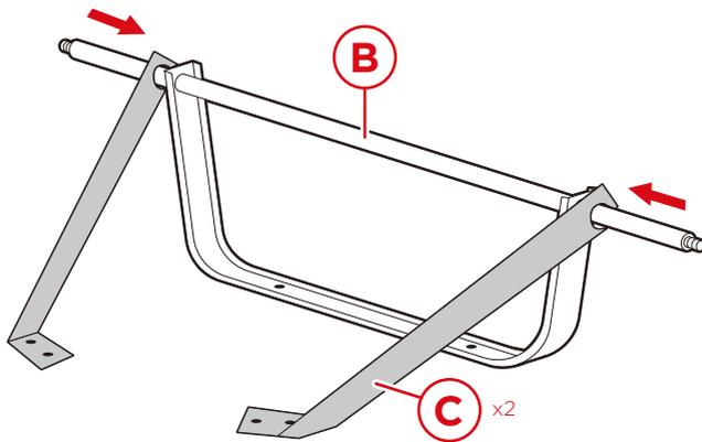
Attach part C rear struts to both ends of part B rear axle frame.
