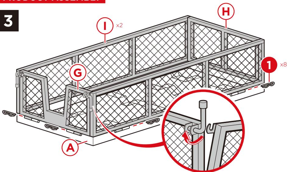
Attach part G front panel, part I side panels, and part H rear panel to part A bottom frame using two part 1 B pins for each panel.
