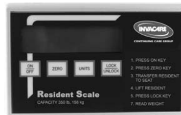
FIGURE 2.4 Using the Scale (Model 1900S ONLY)
