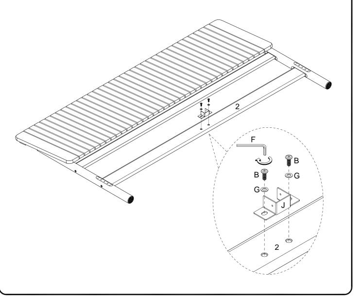
Repeat that process on the Bottom Rail (7) to attach the other U bracket (J).
