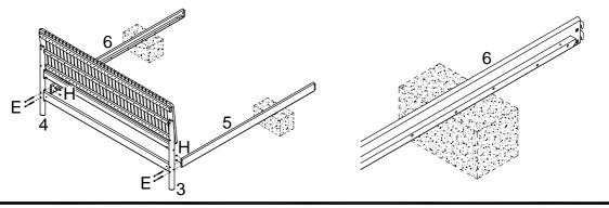
Attach the Bottom rail (7) to the Side rails (5 & 6) by lifting the hooks into the slots and then locking them down into place.
