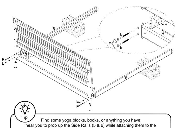
Find some yoga blocks, books, or anything you have near you to prop up the Side Rails (5 & 6) while attaching them to the Headboard Posts (3 & 4). Insert the Bolts (E) through the backside of the Headboard Posts (3 & 4) and thread them into the Barrel nuts (H) until tight.
