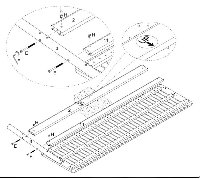
Repeat that process on the other side of the Headboard (1), attaching the Right Headboard Post (4) to the Bottom Headboard Support Rail (2) and Middle Headboard Support Rail (11) with the Bolts (E) threading into the Barrel Nuts (H).
