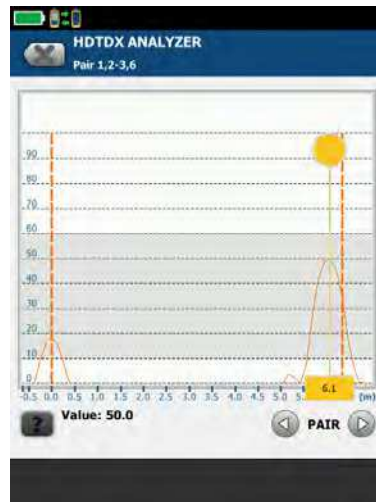
High Definition Time Domain Cross talk (HTDTC) shows the far end connection is clearly the issue
