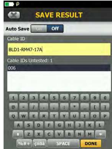
Quickly enter Cable Ids with the capacitive touchscreen
