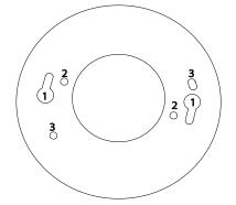
6 For keyholes: Pre-install screws into J-Box and align keyhole slots to screws. Press fixture into box. For all others press fixture into box, then install screws.
