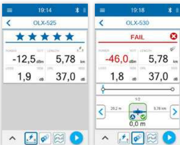
Figure 3. Optical Explorer displays power, length, loss and ORL in combined view.
