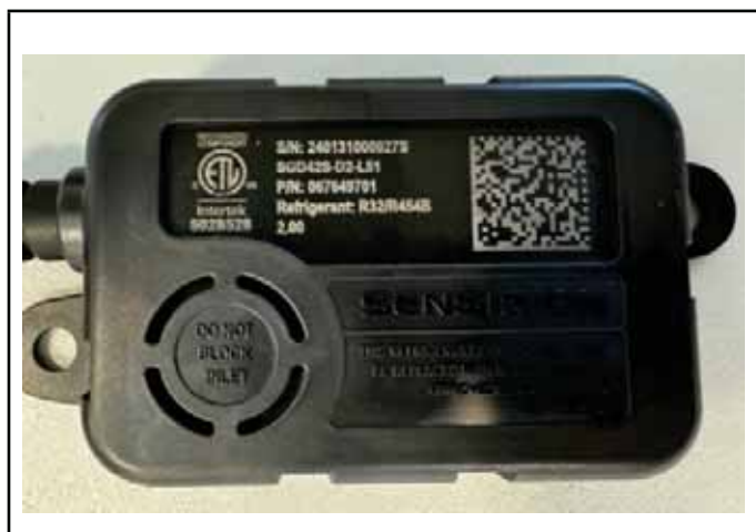
Figure 29. Example of Clear, Unobstructed Sensor Inlet
