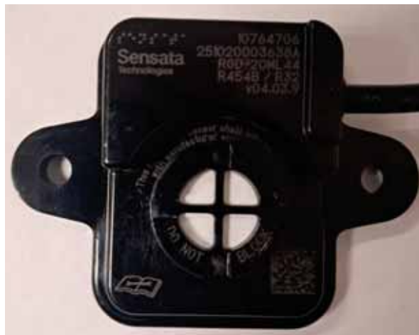
Figure 30. Example of Clear, Unobstructed Sensor Inlet
