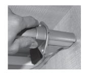
**2.** If the profile needs to be trimmed down in length, use a chop or hacksaw to cut to proper length. Deburr all cut edges.
