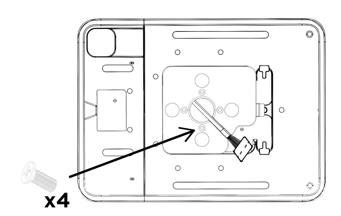
16. Plug the molex connector from the Mount into the cable on the CONNECT CASE. Note the gold pins are facing outward when connecting into the Mount cable. Press the Mount cable into the channel to hold and secure the cable out of the way of the iPad.
