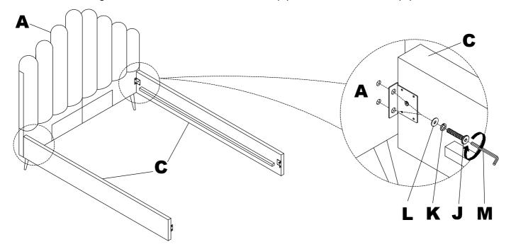
Attach Side Rail (C) to Footboard (B) by using Allen Bolt (J), Spring Washer (K) and Flat Washer (L) and tightening with Allen Key (M).
