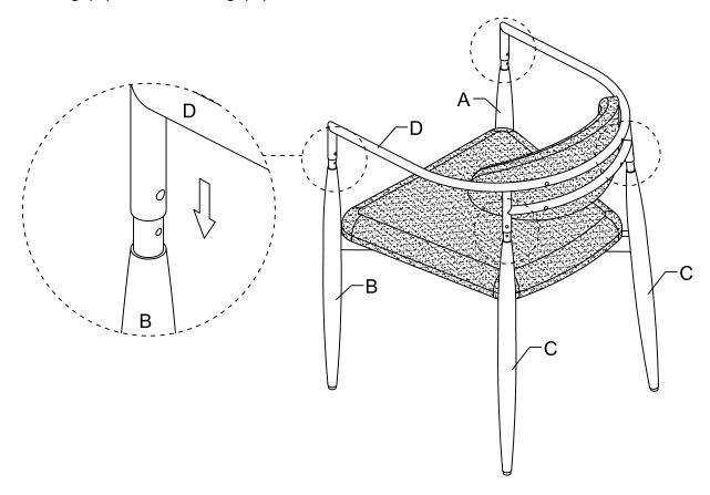
Tighten Arm & Back Rest (D), Left Leg (A), Right Leg (B) and Back Leg (C) by Bolt (H) and Screwdriver (Not Provided).
