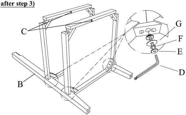
2 Attach the other Leg (B) to Shelf (C) using JCBC Bolt (E), Spring Washer (F) and Flat Washer (G).
