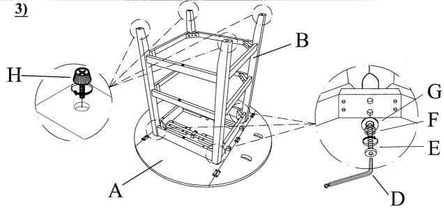
4 Stand table up on the flat surface and check that it is balanced. If there is slight wobble, please adjust the leveler. Lift up the leaf and pull out the wood support which underneath of table top till fixed and tight.
