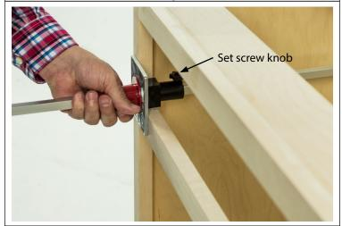
Keeping pressure on aluminum rod and bracket, tighten set screw knob for quicker installations of same cabinet depth.
