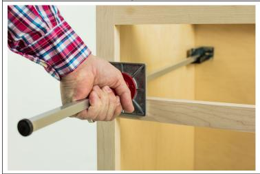
Making sure slide bracket is firmly attached to end of tool, carefully extend aluminum rod to back of cabinet with other hand.
