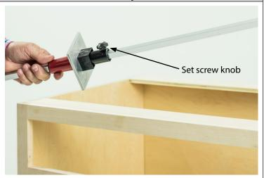
Make sure set screw knob is facing upward. Loosen set screw.
