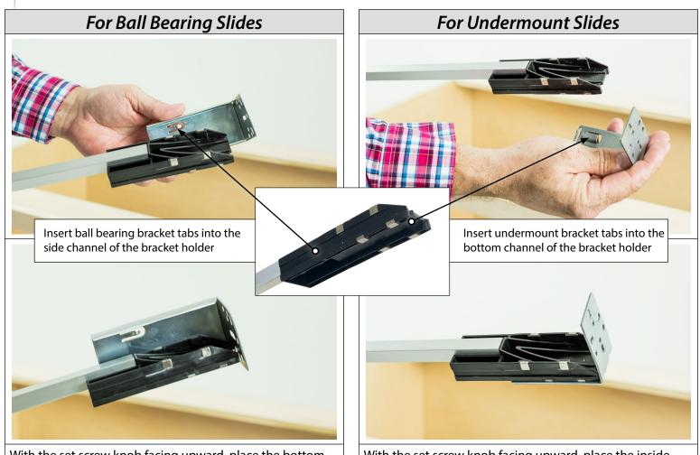
With the set screw knob facing upward, place the bottom of the magnetic bracket holder into the bottom channel of slide bracket. Make sure the bracket is square and pushed firmly against end of bracket holder. With the set screw knob facing upward, place the inside bottom of the slide bracket against the bottom of the magnetic bracket holder. Make sure the bracket is square and pushed firmly against end of magnetic bracket holder.
