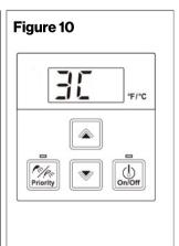
5. When "3C" appears on the display, press and hold button "A" for 5 seconds (Figure 11).
