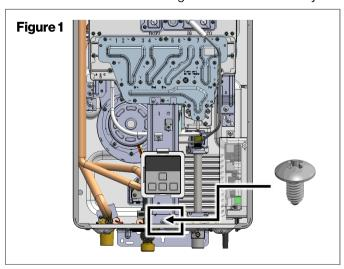
6. Position the controller to gain access to the ignitor assembly.
