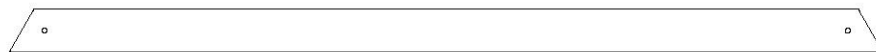
H01 | LISSE DE PLANCHER - W4L15734 (x1) | 1 po x 3 3/8 po x 68 1/2 po (24x86x1741)
