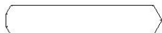
H10 | PLANCHE DU PIGNON - W4L15986 (x2) | 1 po x 3 3/8 po x 17 3/8 po (24x86x440)
