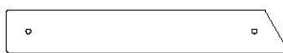
H02 | LISSE DE PLANCHER - W4L15735 (x2) | 1 po x 3 3/8 po x 22 1/8 po (24x86x564)
