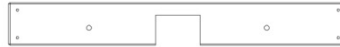
H19 | RAIL DE SOL DU NID DE CORBEAU - W4L12724 (1) | 1"x3 3/8"x27" (24x86x686)
