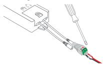
2. Insert Male Plug on Receiver into Female Barrel Connector. Use Flat blade screwdriver to loosen screws on Female Barrel Connector. Insert wires, Red wire to (+), Black wire to (-), and tighten screws. Insert the other end of wires into EZ-WSC Connector.
