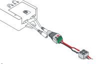
**3.** Use #1 Phillips to loosen the 4 terminal screws on 8MM-EZ Connector. Peel 1/2" of the adhesive protector from back of LED tape light, insert into connector, evenly tighten screws. Insert wires from Receiver into terminals, Red wire to (+) side of tape, Black wire to (-) side of tape; tighten screws.
