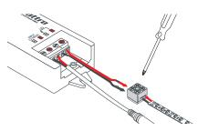
**5.** Use #1 Phillips to loosen the 4 terminal screws on 8MM-EZ Connector. Peel 1/2" of the adhesive protector from back of LED tape light, insert into connector, evenly tighten screws. Insert wires from Receiver into terminals, Red wire to (+) side of tape, Black wire to (-) side of tape; tighten screws.
