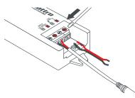
**4.** Insert one end of stripped wires into Receiver LED terminals, Red wire to (+) and Black wire to (-) terminals. Tighten screws.
