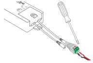
**2.** Insert Male Plug on Receiver into Female Barrel Connector. Use Flat blade screwdriver to loosen screws on Female Barrel Connector. Insert wires, Red wire to (+), Black wire to (-), and tighten screws.
