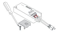
**2.** Use #2 Phillips to loosen screw and remove cover from Receiver.
