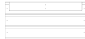
WP7 | CLOISON CENTRALE ARRIÈRE SUPÉRIEURE - W2A02989 (x1) 1 1/2"x21 1/8"x9 3/4" (38x536x248)
