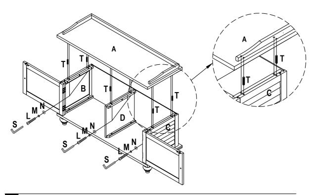
Put Seat Cushion (K) into Top Panel (A) as drawing below and then adjust the levelers on the bottom of the Middle Leg (J) to keep the level.
