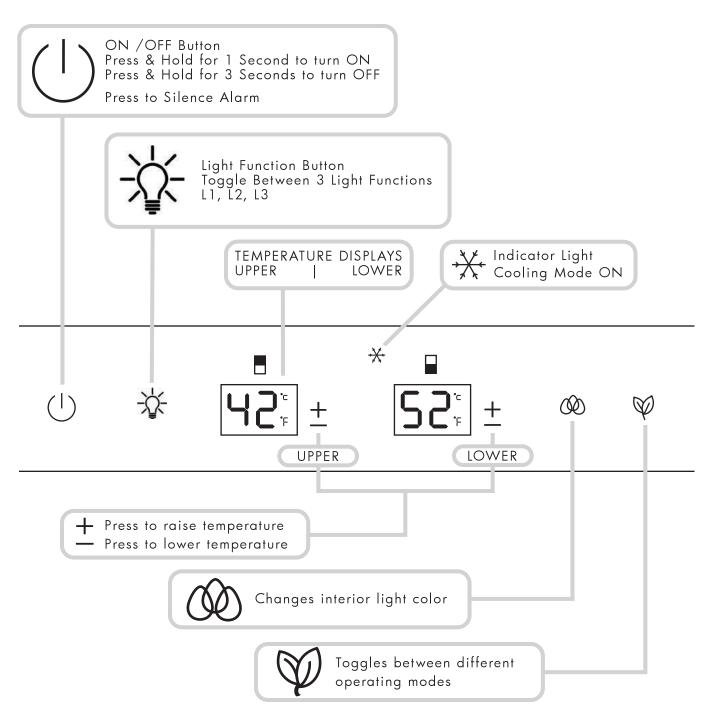
Upper compartment:The temperature setting can be adjusted from 41-50°F. Lower compartment:The temperature setting can be adjusted from 50-64°F. Your controls are simple and intuitive to operate.
