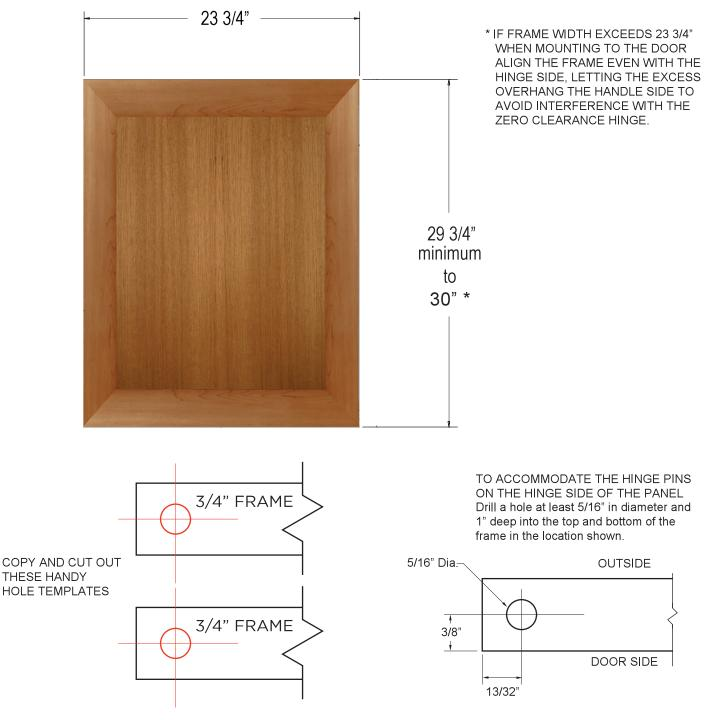
AFTER INSTALLATION UNDERCOUNTER, OVERLAY DOOR MUST BE ABLE TO OPEN 90°.
