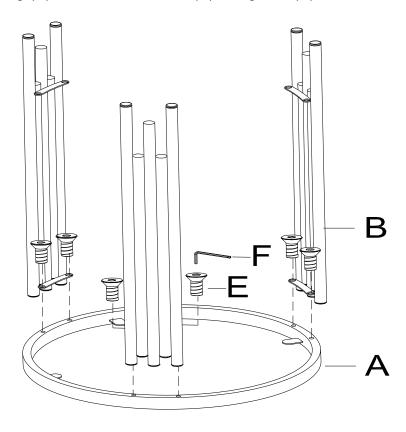
Attach the other Table Frame (A) to the Leg (B) using Bolt (E) with Allen Wrench (F).
