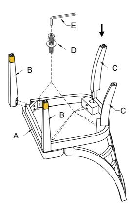
Take the Allen Key and turn the bolts until the legs are secured. DO NOT TIGHTEN THE BOLTS COMPLETELY. Stop when you feel you are adding force to tighten the bolts.
