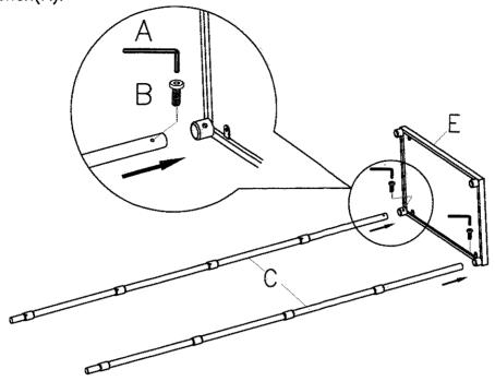
2 Assembly the Shelf Panel(F) onto the Leg Left & Right(C), then using the Bolt(B) by Allen Wrench(A).
