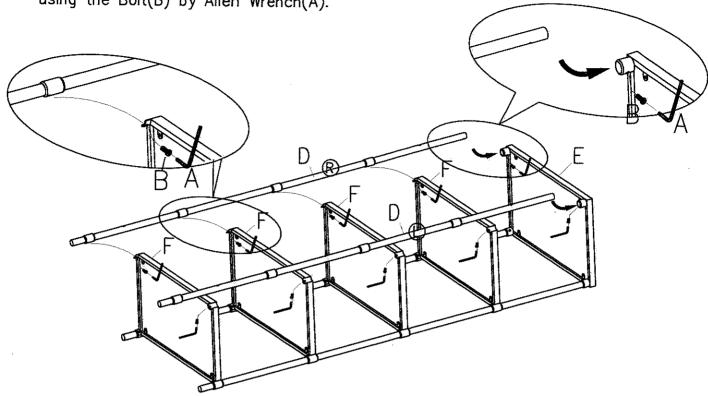
Assembly the Cross Bar(G) onto the Leg Left & Right(D), then using the Bolt(B) by Allen Wrench(A).
