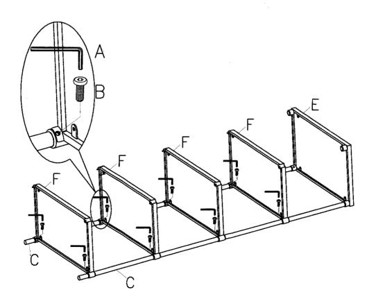
Assembly the Leg Left & Right(D) onto the Top Panel(E) and Shelf Panel(F), then using the Bolt(B) by Allen Wrench(A).
