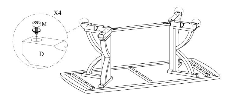
7 Stand the table on an even surface and check for balance. If the table wobbles slightly, please adjust the Leveler (M).
