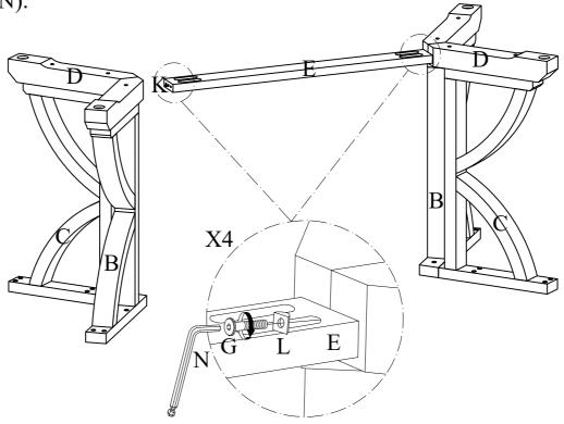
5 Place the Table Top (A) upside down on an even surface. Align and attach the Leg Frame (B & C) to the Table Top (A) using JCBC Bolt (F) and Lock Washer (I) and Flat Washer (J) with the Allen Wrench (N).
