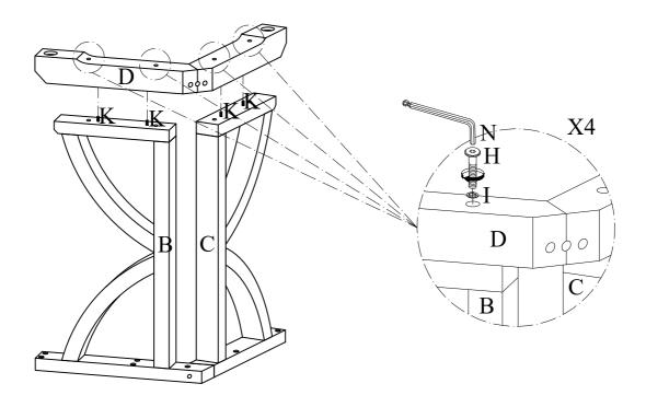
4 Use PVC Dowel (K) as a guide to align and attach the Crossbar (E) to the Leg Base (D) using JCBC Bolt (G) and Nylon Washer (L) with the Allen Wrench (N).
