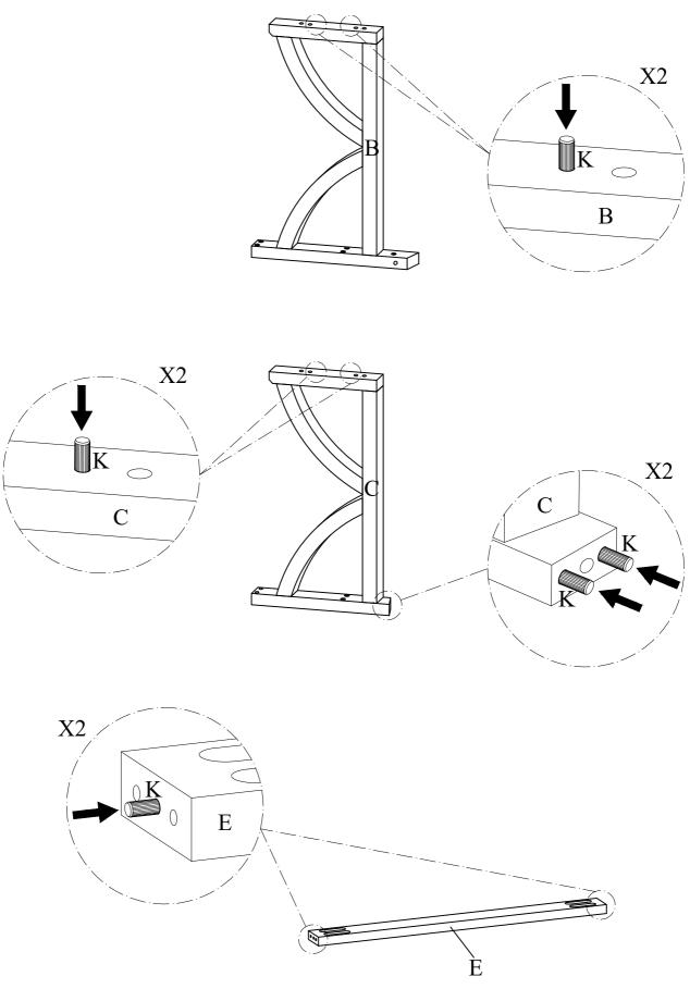
2 Use PVC Dowel (K) as a guide to align and attach the Leg Frame (B) to the Leg Frame (C) using JCBC Bolt (H) and Lock Washer (I) with the Allen Wrench (N).
