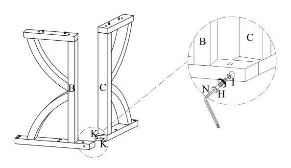
3 Use PVC Dowel (K) as a guide to align and attach the Leg Base (D) to the Leg Frame (B & C) using JCBC Bolt (H) and Lock Washer (I) with the Allen Wrench (N).
