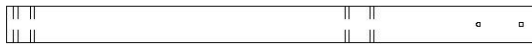
SP01 | SOPORTE DE LA VIGA DEL COLUMPIO - W4L16462 (x1) 3 3/8"x3 3/8"x50" (86x86x1269)
