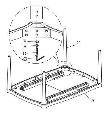
**2** Turn the Table upright on a flat surface so that the Table will not wobble. Tighten all Allen Bolt (D) by using Allen Key (G). Unlock the sash locks underneath the Table Top (A).
