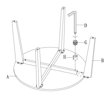
Lock the Leg (B) to the back of the Top Panel (A) by using Bolts (C) with Allen Key (D). Repeat step 1 and step 2 to assemble other 3 legs.
