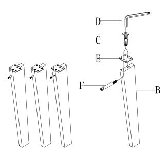
Put Cam Nut (H) on the back of Top Panel (A), then put the Leg (B) closed to the Cam Nut (H). Lock the Cam Screw (G) by using Allen Key (D).
