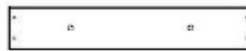
H110 | PLANCHE DE FIXATION - W4L14946 (x1) | 1 po x 3 3/8 po x 19 1/4 po (24 x 86 x 488)
