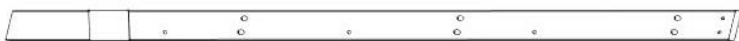
H04 SOLIVE DE TOIT - W4L16784 (x1) 15/16 po x 3 3/8 po x 85 3/4 po (24x86x2203)
