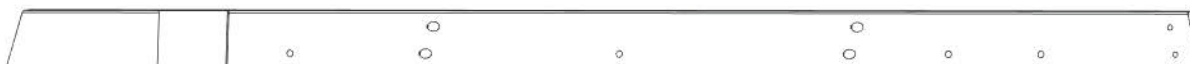
H12 SOLIVE DE TOIT - W4L16802 (x2) 15/16 po x 3 3/8 po x 79 1/4 po (24x86x2013)
