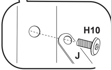
\* Make sure the mattress support board (J-1&J-2) is installed **FLAT SIDE UP**.
