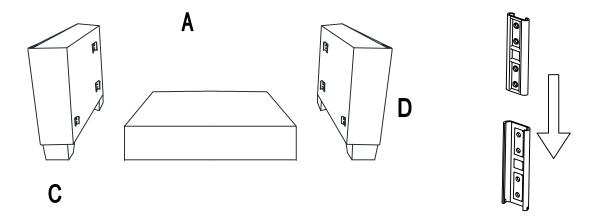
Hook on the Back Frame (B) to Left Panel (C) & Right Panel (D) properly.
