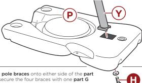
Locate and overlap the four part U pole braces onto either side of the part Y lower pole's fastener hole, then secure the four braces with one part G bolt & nut set.
