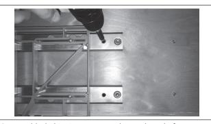
Remove black shipping screws as shown above before beginning installation
