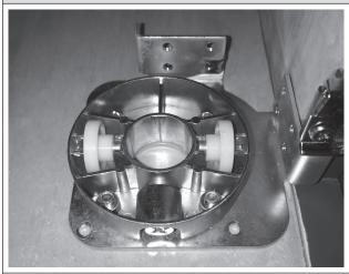
Place the Lower Hub Assembly tight against the back corner of the face frame (the panel divider in frameless applications) and firmly secure with 4 four #8 X 5/8" Pan Head Phillips Wood screws provided as shown above.
