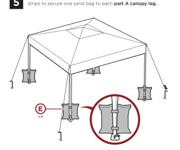
Fill four part E sandbags with clean sand, then use the self-adhering
